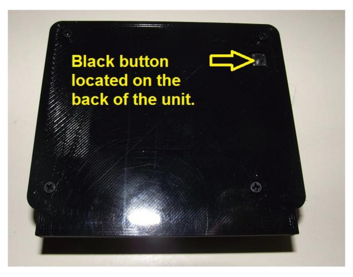
On the back of the touchscreen scan tool, you will find a black button, hold this button down during power up. If you did this successfully the screen will be a solid white color, and the unit is then waiting for a software update. Plug a USB mini cable (commonly found on dash camera, some cameras, tablet, or older cell phone) to the side of the unit and attach to your Windows PC. Use Windows device manager to verify that you have a valid USB Serial driver Ports (COM & LPT).
