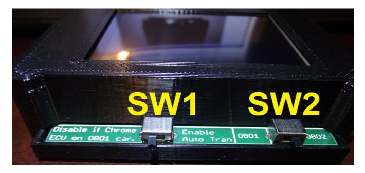
Whenever you switch from an OBD1 car (1991-1993) to OBD2/MUT car (1994-1999) you will have to move the switch (SW2) to the corresponding type. The software will remind you to adjust this switch when connecting to the engine ECU.
