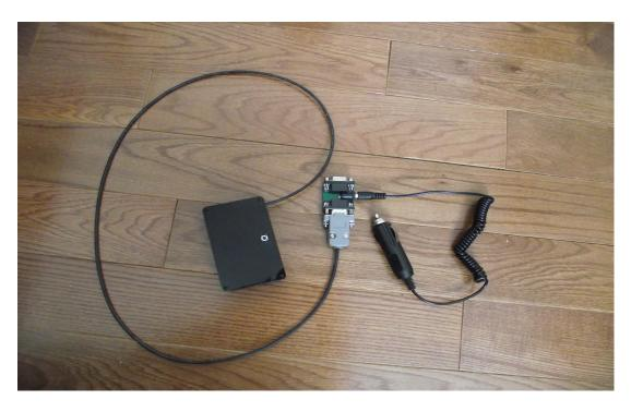
You will most likely require a USB-to-serial adapter if your notebook does not a have serial connector. On the back of the touchscreen scantool, you will find a black button, hold this button down during power up. If you did this successfully the screen will be white, and the unit is then waiting for a software update.
